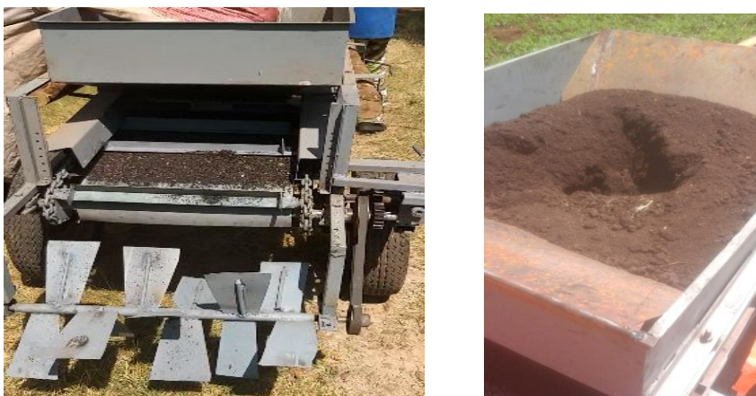
Fig 1. The Manure applicatormachine (left), the hopper part filled with manure
