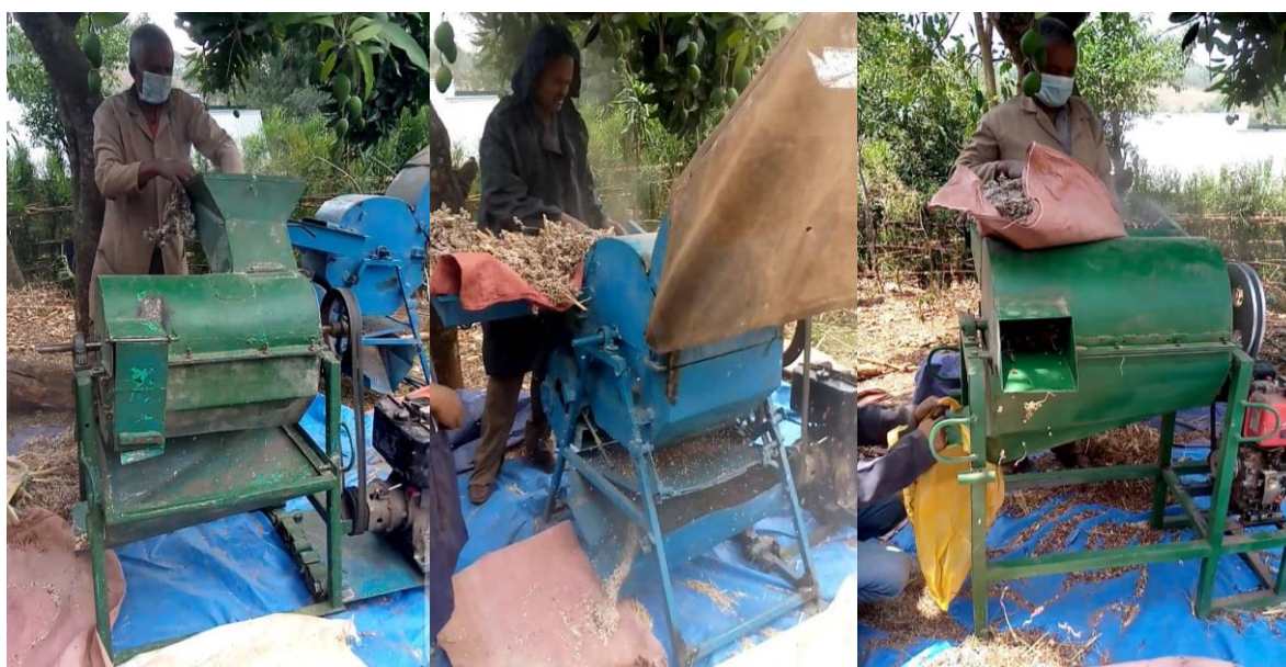
Fig.1.a. Jimma Replaceable Drum Multi Crop Thresher b. Jimma Rice Thresher c. Fadis Sorghum thresher
