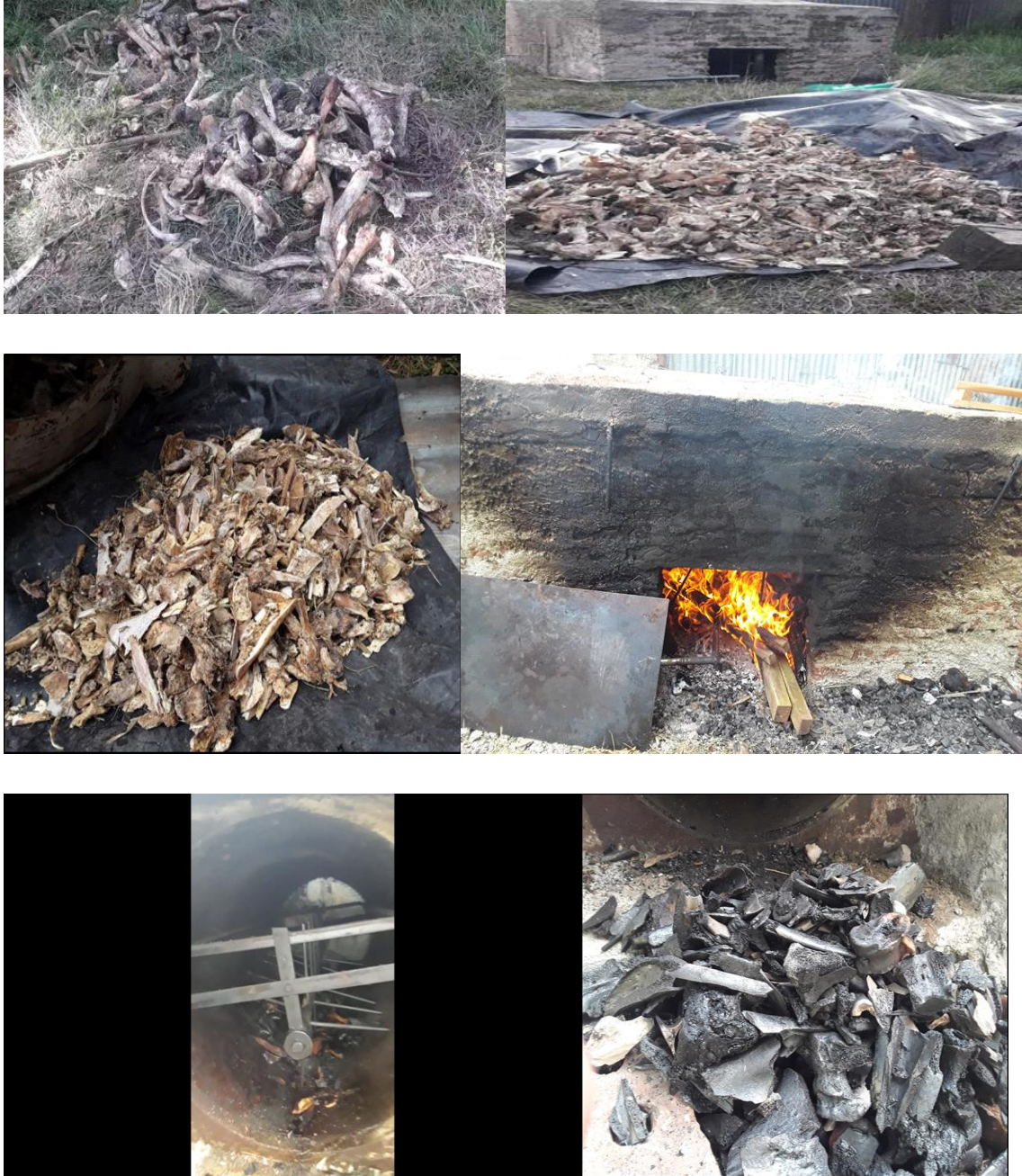
Figure 1: Steps to produce bone char using pyrolysis kiln
