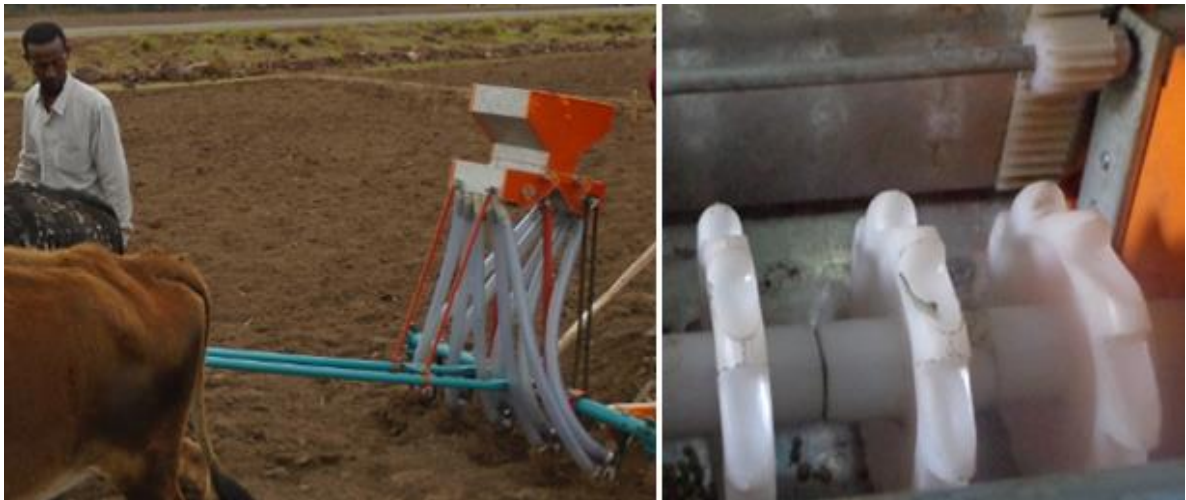
Figure 1. a. Dharti seed cum fertilizer row plant at field b. seed metering roller
